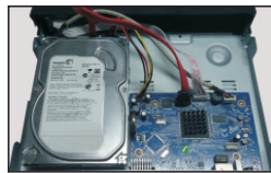
④ Place the HDD onto the bottom of the machine.
