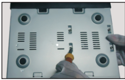
⑤ Turn over the machine and secure the HDD with the screws.
