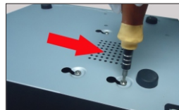
④ Turn over the machine and secure the HDD with the screws.
